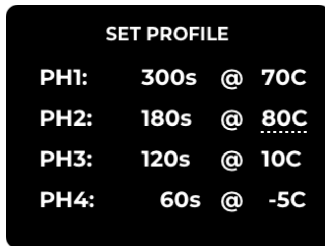
Figure 7. Set Profile screen. The underlined field is the field currently being edited; it blinks on the live display.
