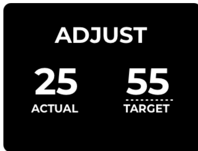
Figure 6. Adjust mode; the underlined TARGET digits blink while the value is being edited.
